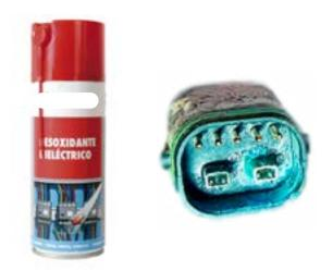
When electrical connections come into contact with damp spots or are clogged due to external contamination, a chemical reaction occurs, causing a build-up of lead sulphate crystals in the connections. In other words, the copper on the contacts will rust, resulting in conductivity problems.
