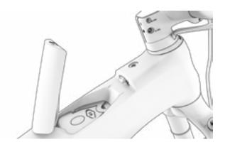
3. LIFT THE BATTERY HANDLE AND PULL UPWARDS TO CHARGE IT OUTSIDE THE FRAME.
