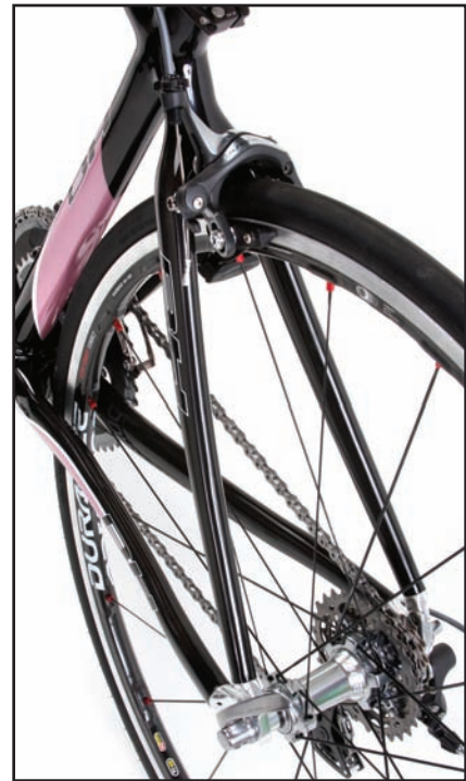
Rear stays are manipulated to provide a compliant ride.
