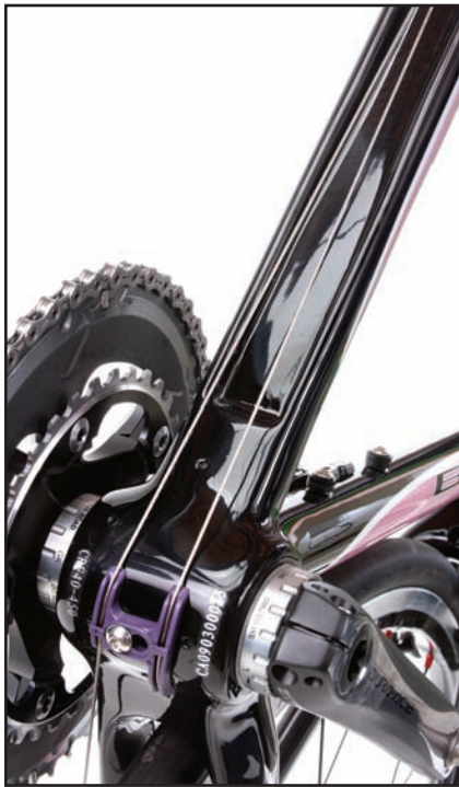
The BH downtube channel has Di2 battery mounts.
