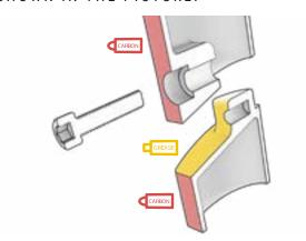
3. INSERT THE SEAT POST INTO THE FRAME AT THE DESIRED HEIGHT AND TIGHTEN THE BOLT.
