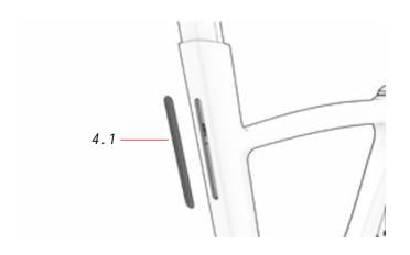
Always observe the specified maximum and minimum heights to ensure that the integrated seatpost clamping system functions correctly. Damage resulting from incorrect adjustment will not be covered by the warranty and could lead to serious accidents.
