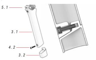
▲ Bolt 4.2 must be inside the seat post and parts 3.1 and 3.2 aligned.
