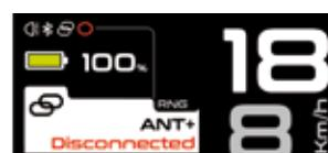
Ant+ Connected/Disconnected notification
