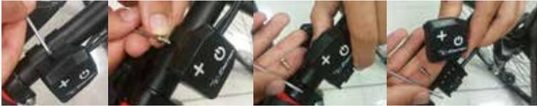
**NOTE** In order to reduce risk of theft, to remove (or insert) the panel screw, the user must first loosen the grips, left brake lever, shift lever and the panel support bracket.
