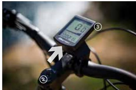
**2. Switching the Pedal Assistance System on and off.**
