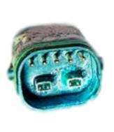
When electrical connections come into contact with damp spots or are clogged due to external contamination, a chemical reaction occurs, causing a build-up of lead sulphate crystals in the connections. In other words, the copper on the contacts will rust, resulting in conductivity problems.
