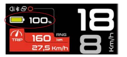
The range of the system will vary depending on the following riding conditions, among others: frequent starts and stops, transmission ratio, numerous steep slopes, road surface in poor condition, carrying heavy loads, strong wind coming towards the cyclist, low temperatures, degradation of the battery, use of the built-in lighting system, incorrect tyre pressure, chain or brake settings.
