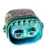
When electrical connections come into contact with damp spots or are clogged due to external contamination, a chemical reaction occurs, causing a build-up of lead sulphate crystals in the connections. In other words, the copper on the contacts will rust, resulting in conductivity problems.
