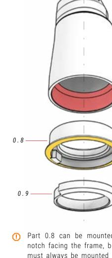
Part 0.8 can be mounted with the notch facing the frame, but part 0.9 must always be mounted in the first position, as shown in the images.
