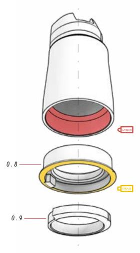
1 Part 0.8 can be mounted with the notch facing the frame, but part 0.9 must always be mounted in the first position, as shown in the images.
