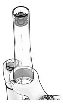
⚠ It is recommended to use a duller to ensure that the spider is inserted into the steerer tube perfectly aligned.
