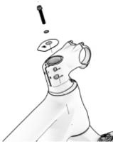
THE 4. IF YOU DO NOT REMOVE THE WASHERS, TIGHTEN BOLT "I" FIRST AND THEN BOLT "II". TO REMOVE THE STEM, START BY REMOVING BOLT "II".
