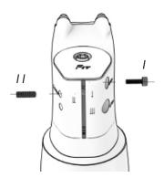
▲ The purpose of tightening the bolts is to keep the washers from moving. Therefore, do not apply too much torque.
