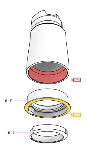
() Part 0.8 can be mounted with the notch facing the frame, but part 0.9 must always be mounted in the first position, as shown in the images.
