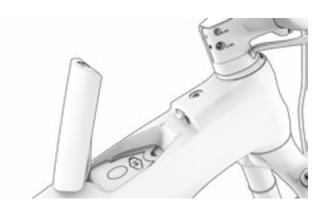
3. LIFT THE BATTERY HANDLE AND PULL UPWARDS TO CHARGE IT OUTSIDE THE FRAME. LEAVE IT IN PLACE IF YOU WISH TO CHARGE IT INSIDE THE FRAME.
