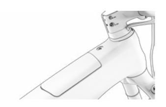
5. OPEN THE BATTERY COVER TO CONNECT THE BATTERY CHARGER FIRST AND THEN PLUG INTO THE POWER SOCKET.
