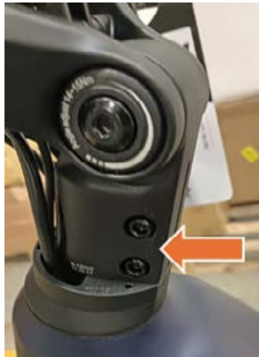
4. TIGHTEN THE SCREWS TO 9-10 NM
