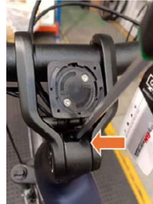
3. ADJUST THE SCREW TO REDUCE THE GAP
