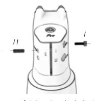
⚠ The purpose of tightening the bolts is to keep the washers from moving. Therefore, do not apply too much torque.
