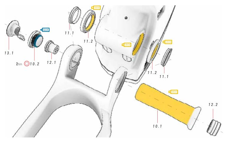
1 The maximum tightening torque of part 10.2 is 2 Nm, since it is designed to prevent gaps. Bolt 12.2 will secure part 10.2 and the remaining swingarm assembly.
