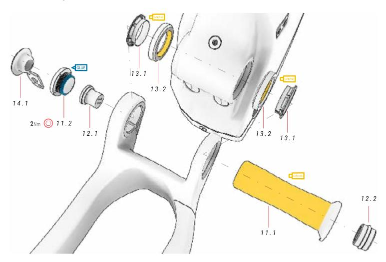
The maximum tightening torque of part 11.2 is 2 Nm, since it is designed to prevent gaps. Bolt 10.2 will secure part 11.2 and the remaining swingarm assembly.
