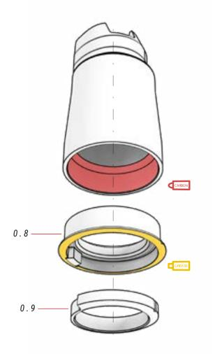
Part 0.8 can be mounted with the notch facing the frame, but part 0.9 must always be mounted in the first position, as shown in the images.
