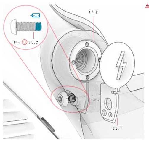
↑ Always loosen bolt 10.2 before mounting or dismounting part 11.2. Part 11.2 has been designed so it can be threaded or removed with a "Pin Spanner" or similar tool. 2.4 mm hole diameter.
