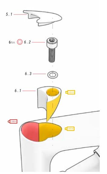
STANDARD CLAMP ON ALLOY MODELS: EC826 / EC816 / EC806 / EC796
