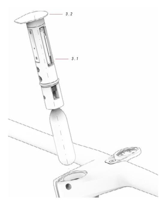
! The headset must be completely empty inside before the FIT tool can be fitted. Use the FIT washer system designed for this purpose and remove any obstacles such as the spider on the head tube.
