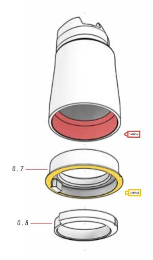
Part 0.7 can be mounted with the notch facing the frame, but part 0.8 must always be mounted in the first position, as shown in the images.
