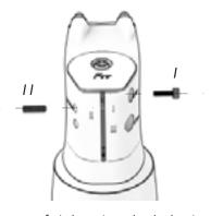
⚠ The purpose of tightening the bolts is to keep the washers from moving. Therefore, do not apply too much torque.
