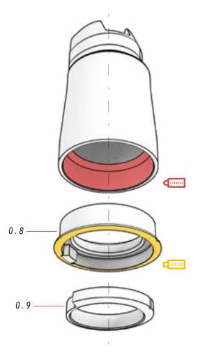
Part 0.8 can be mounted with the notch facing the frame, but part 0.9 must always be mounted in the first position, as shown in the images.
