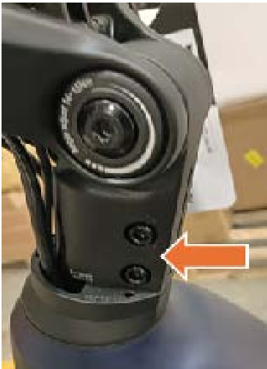
4.TIGHTEN THE SCREWS TO 9-10 NM
