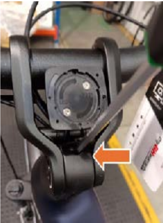
3. ADJUST THE SCREW TO REDUCE THE GAP.
