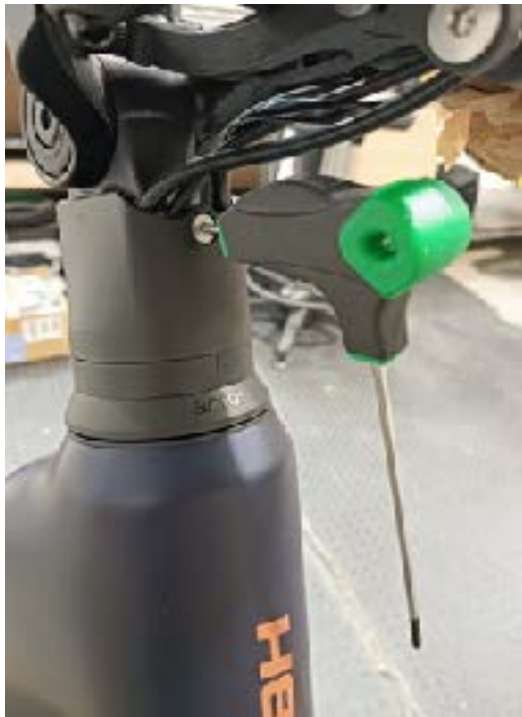
1. REMOVING THE STEM COVER.
