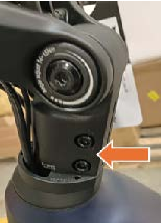
2. LOOSEN THE STEM SCREWS.
