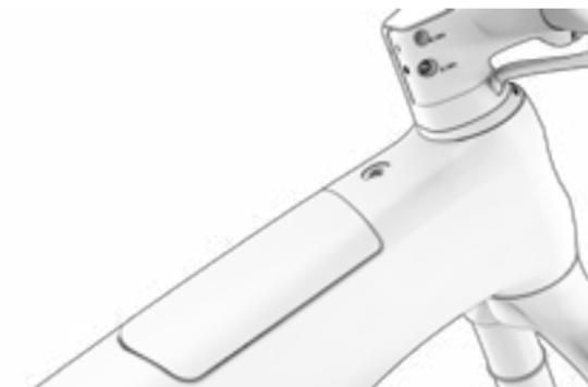
5. OUVREZ LE COUVERCLE DE LA BATTERIE POUR CONNECTER LE CHARGEUR DE BATTERIE D'ABORD, PUIS BRANCHEZ-LE SUR LA PRISE D'ALIMENTATION.
