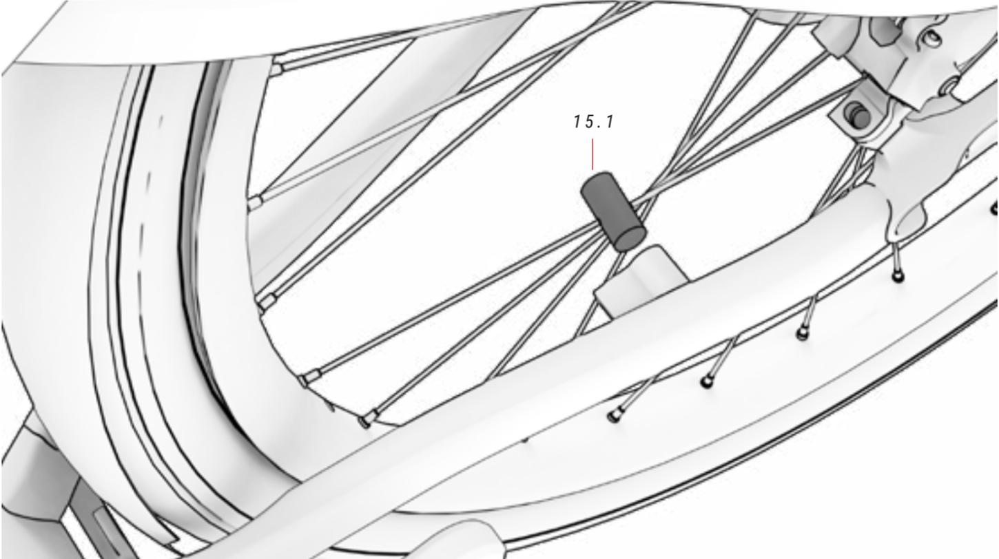
**15** MAGNETO SENSORE VELOCITÀ *ref. Shimano spare part*
