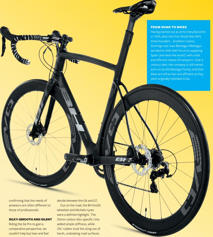
Riding the G6 Pro to gain a comparative perspective, we couldn't help but hear and feel the rear brake blocks rubbing against the rim when standing; a common (but agonising) downside to many rear brakes mounted beneath the chainstays. But when out of the saddle on the G7, the disc brakes were silkily silent – which could be a decisive difference if you can't
