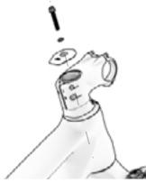
E THE 4. IF YOU DO NOT REMOVE THE WASHERS, TIGHTEN BOLT "I" FIRST AND THEN BOLT "II". TO REMOVE THE STEM, START BY REMOVING BOLT "II".
